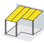
Pent roof with roof guttering offset
